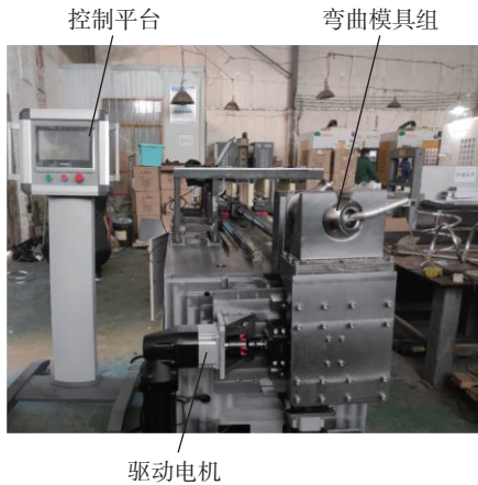
图 28 管件弯曲试验设备 Fig.28 Tube bending test equipment
